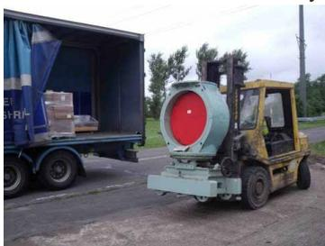
Removal of the mirror from the control room of the tunnel - now a seriously derelict building - was hampered by its 2.5 tonne weight and the need to manhandle it to a loading bay some 50 metres away across wooden flooring and piles of brick rubble. Movement was managed using 6ft crowbars to inch it over steel plates laid to form a pathway over the roughest areas. The loading bay doors also presented a difficulty as they had been closed for 30 years or so and the
