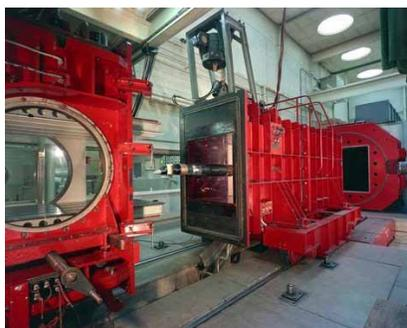
3x3 tunnel showing model in working section, 1967 [CL203]
