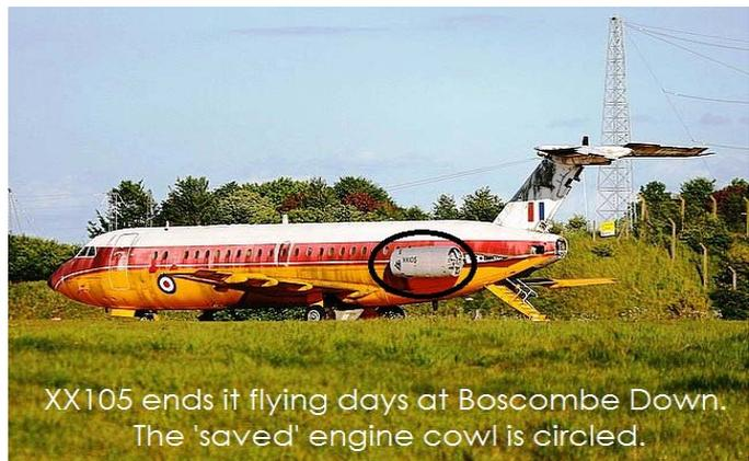
XX105 ends its flying days at Boscombe Down. The ‘saved’ engine cowl is circled.
