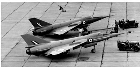
the BAC221, as part of the Concorde research programme. This was then delivered back to Bedford from Filton by RAE test pilot Clive Rustin on 20 May 1966. The picture (right) is a rare shot of the two aircraft airborne together, and shows clearly 774's new ogival wing shape appropriate to Concorde.
