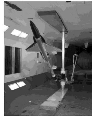
*High Incidence Research Model (Model 2061 HIRM-LERX) on sting rig 13x9 1978 (neg C20797)*
