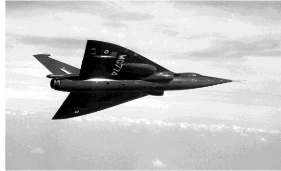
BAC 221 showing Concorde-like ogee wing shape (neg B2495C)
