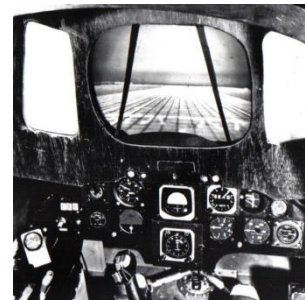
Simulator cockpit showing runway using TV technology (neg B3029)
