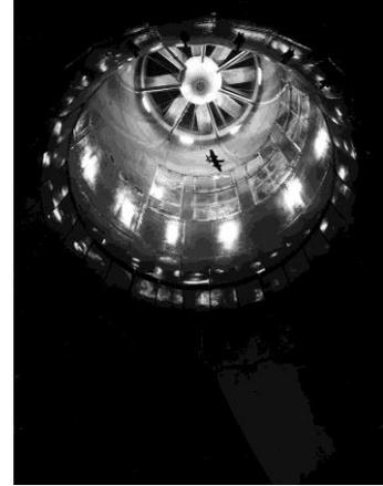
*The Vertical Spinning Tunnel and associated buildings (neg CL839, 1982) Meteor model under test in VST (neg M244 EH35 37895-34)*
