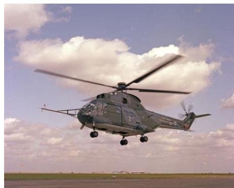
Puma XW241 airborne, showing the vanes for airflow measurements mounted on a nose boom (neg B6040D 1982)
