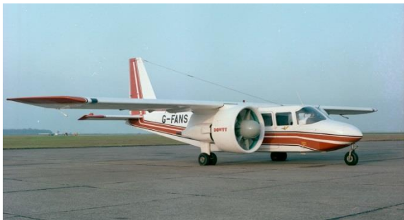
Britten Norman Islander G-FANS with Dowty Ducted Fan engines, Nov 1979 (neg B5182F)
