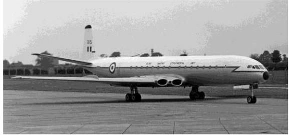
My first flight on XP915, as a Flight Test Observer, was on 11 September 1968, investigating new autoland control laws. For this, we used a PACE TR 48 analogue computer, the only practical solution at the time, as digital computers were too large for the aircraft cabin, and also too slow in response time.
