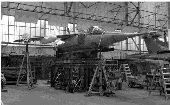
on a special rig in the hangar (see picture, neg B4705A, May 1978) in order to measure its moments of inertia. Differences from the aircraft manufacturer's predictions helped explain discrepancies between flight and wind tunnel measured values of stability and control parameters. The Gnat was also used to explore the phenomenon of "wing rock", consisting of sustained or even divergent roll oscillations, a form of
