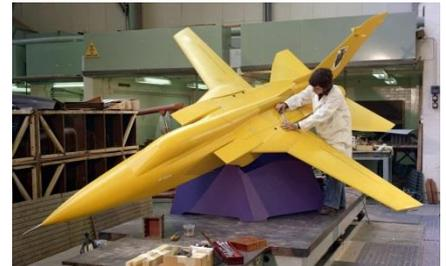
flying drop models (Tornado, *neg CL536, 1978*). Depending on the size of the real aircraft, wind tunnel models were typically made at a scale of 1:30 or 1:36. Specialised and complex highly-detailed models, such as Concorde air intakes, below, right (*neg C8976, 1964*), were made at other scales. Models were also made with variable configurations of stores – weapons and drop tanks – as in the heading picture of a Tornado model.
