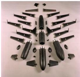
All models had to be finished to a high degree of accuracy, to avoid any blemish on the model that might distort the results. Typically this involved machining to a thousandth of an inch. For some trials, models were made as a “kit of parts” so that a range of alternative configurations could be tested (see picture
