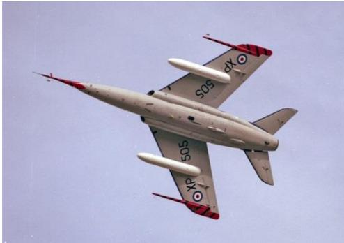
Gnat XP505 (neg B4849E, Oct 1978, pilot Flt Lt George Ellis) showing air data probes at wing-tips and on the nose
