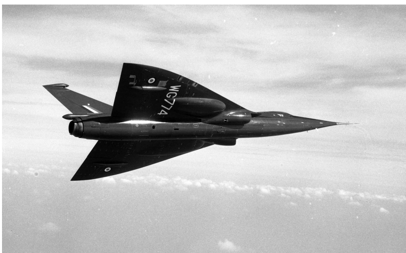
BAC 221 supersonic research aircraft tested at RAE Bedford, showing Concorde-like "Ogee" wing
